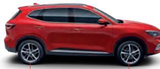
Wheelbase 2720mm Length 4574mm
